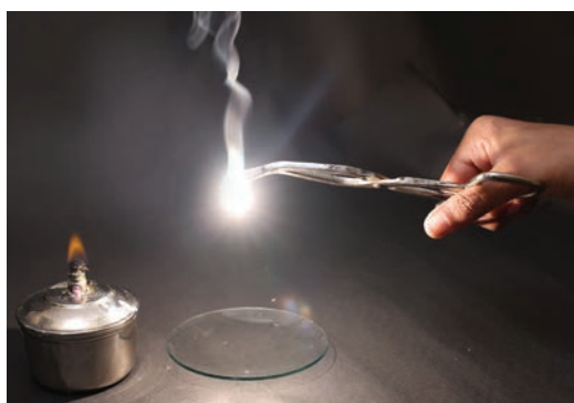
Fig. 5.5: Burning magnesium ribbon
